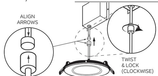
**STEP 8 ->** Insert junction box through the mounting hole
