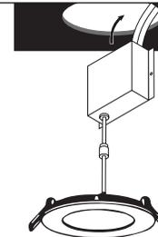
**STEP 9 ->** (Applies when an additional trim is used to change the color of the finish. If this does not apply, go to step 10)
