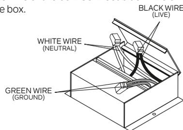
**STEP 7 ->** Join both white cables in order to affix the slim light to the junction box.
