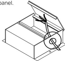
**STEP 4 ->** Insert the electrical cable through the knockout.
