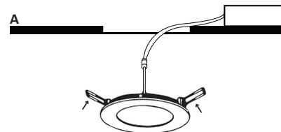
B) Release the clips and the fixture will be pulled flush to the ceiling.
