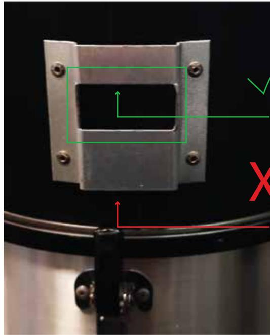
The hook must go through the middle of the bracket.
